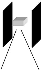
**Poor location:** Narrow window for detection. The signal can't be seen well.
