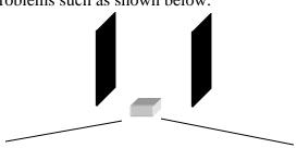
**Good location**: No metal to block the signal. The detection window is very wide.
